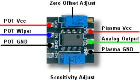
Alternately, the X-Amp can be used to amplify this signal to approx 100% or 1023 steps in Windows. Sensitivity increase is approximately 14 times in this case.
