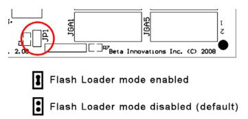
RESET jumper JP1 can be used to restart the device in Flash Loader mode should the module fail to function after an update. It should remain open (disable) for normal device operation. The device can be set in Flash Loader mode when needed in order to update the core NITRO-SLG firmware. The jumper must be removed after successful firmware update prior to rebooting the device. See the Device Manager utility user manual for details on firmware update procedures.
